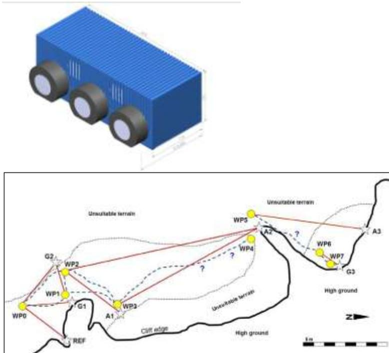
**Figure 1: Early achievements of PRoViScout requirements definition & design work. Left: Dimensional layout of the zoom RGB 3D-TOF camera. © CSEM. Right: Example for waypoints and a globally planned rover trajectory in the area of Clarach Bay (Aberystwyth, UK). © Univ. Leicester.**
